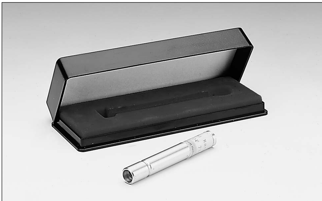
Fig. 1: Source Ra-226, 4.0 kBq in storage-box, 09041.00.
